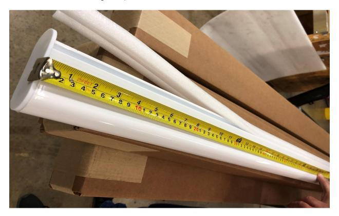
3. Using a Chop (cutting) Saw cut off to desired length.
