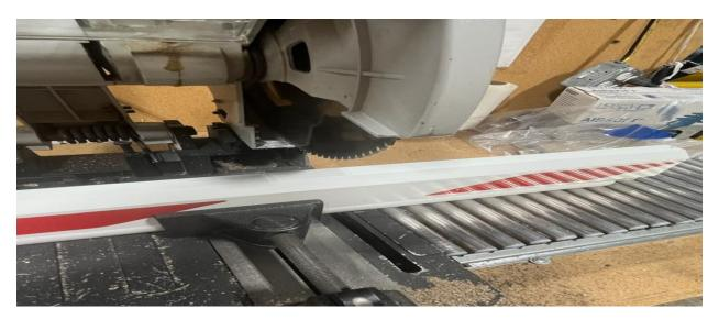
1. On the LED strips, locate copper markings. At the closest marking under the desirable length, cut LED strips on the marking.
